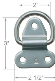
5/16" Hinged Pad Eye Safe Working Load: 1500 lbs
