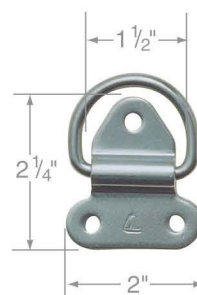
1/4" Hinged Pad Eye Safe Working Load: 1000 lbs
