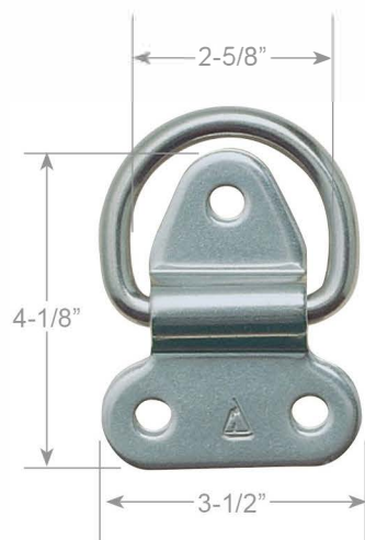
1/2" Hinged Pad Eye Safe Working Load: 3500 lbs
