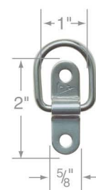
3/16" Hinged Pad Eye Safe Working Load: 400 lbs
