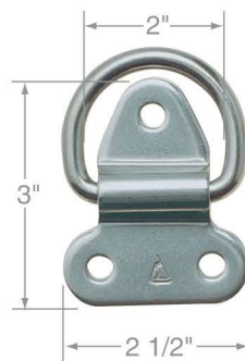
5/16" Hinged Pad Eye Safe Working Load: 1500 lbs
